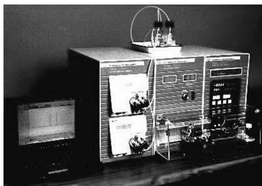
Fig. 1. Photograph of the pressurized gradient capillary electrochromatography (pCEC) instrument.
